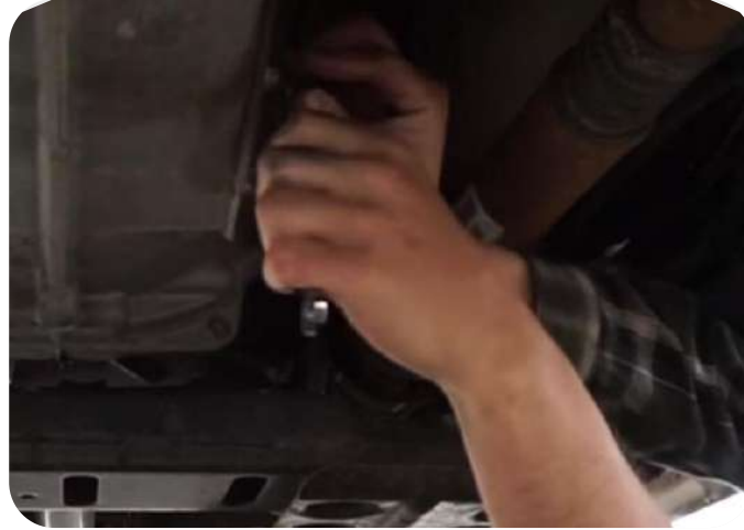
Figure 3- Mounting the PTO on the vehicle
